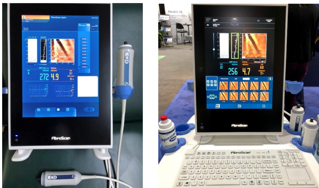
Fig. 5.9 and Fig. 5.10. The FibroScan device, with the two probes M and XL and with the fibrosis (stiffness) module (the result in yellow on the screen) and CAP (the result in blue).
