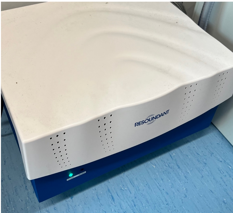
Figure 2 – Active Driver, by Resoundant (Rochester, MN, USA), which is placed outside of the scanning room, which produces waves by pneumatic action
