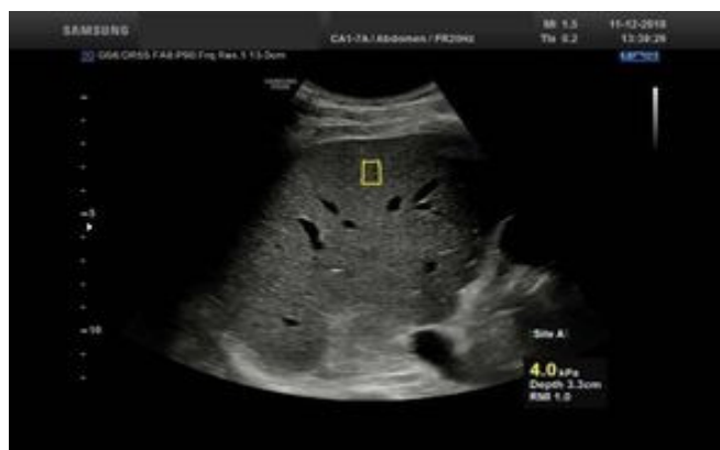
Fig. 5.5. Measurements of liver stiffness using pSWE elastography in a patient without fibrosis (Samsung Medison, South Korea). The region of interest is placed 3.3 cm below the liver capsule, avoiding large vessels. The median (kPa), depth of the region of interest, and RMI (Reliability Measurement Index) are displayed on the screen.
